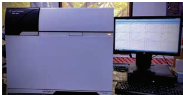
Figure 10 : ICP-MS system, Agilent 7900
